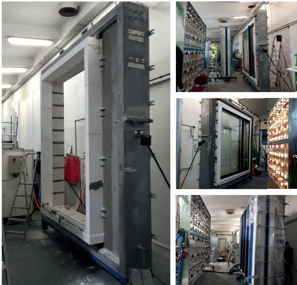
Air-tight and durability testing at ITB Laboratory in Warsaw.
